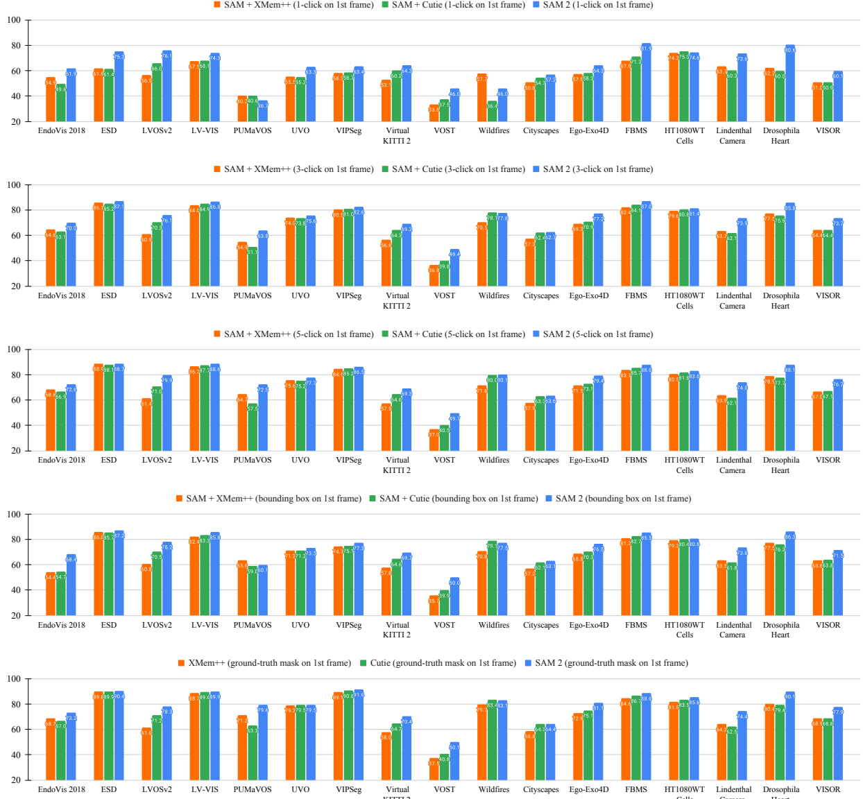
Figure 14 Zero-shot performance on 17 video datasets of SAM 2 vs two baselines (SAM+XMem++ and SAM+Cutie) under semi-supervised VOS evaluation using different prompts (1, 3 or 5 clicks, bounding boxes, or ground-truth masks on the first video frame), with the averaged performance across datasets for each type of prompt shown in Table 4 in the main text. See §F.1.3 for details.
